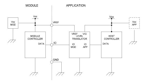
Figure 5.6-1 Typical Level shifter arrangement using VREF
